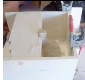
Build your mould box around the other side. Seal edges. Measure, mix and pour the Hydrocal and allow to set.
