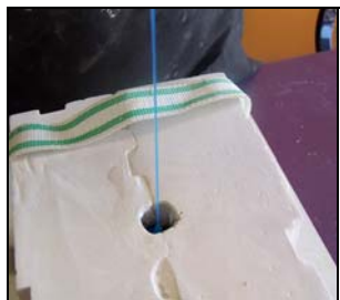
Measure, mix and pour silicone into the jacket through the hole created with clay. Allow silicone to cure
