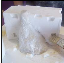
Coat the Hydrocal block with Vaseline (petroleum jelly) to prevent the 2 nd half of the support bonding.
