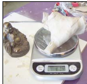
Weigh the clay just taken from the Model. This weight will be approx the amount of silicone required.
