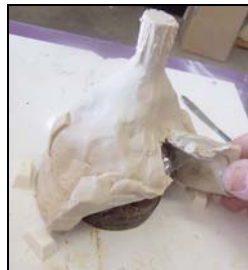
Remove the clay from the Model and put aside, don't discard. Remove the plastic wrap.
