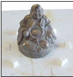
Secure Model and some registration blocks (wood or plastic) to base, approx 25mm outside of Model
