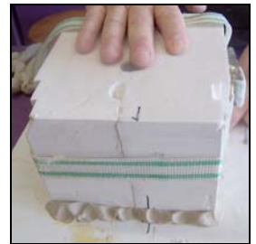
Place the support mould together and hold securely with a strap or tape. Place in position on base board. Seal edges to prevent leakage.
