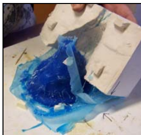
Remove the support jacket, revealing the mould.
