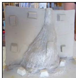
Build separation wall of clay Add clay blocks for registration so that the jacket halves align.
