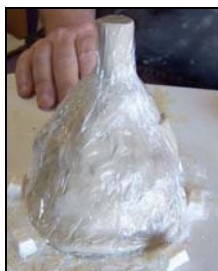
Spray with Vinyl Strip Spray or cover with plastic wrap. Ensure plastic wrap is smooth and registration blocks are well defined
