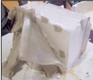
Remove the mould box. Remove the clay from the Hydrocal block, being careful not to disturb the model.
