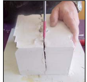
Remove the mould box and use a flat tool (scraper etc) to pry the joint open. Do this slowly so as not to damage any areas.
