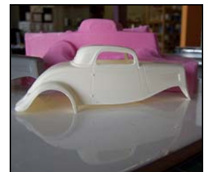
Remove "flash" (thin layer of resin) from edges and other openings.
