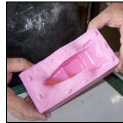
Measure and mix resin. Pour a small amount (about 1/3 of mix) into base mould.
