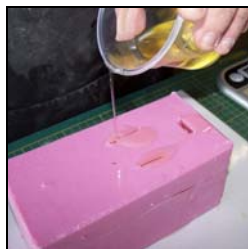
Fill mould with remaining resin. You know mould is full, when resin rises through other air vents. Allow resin to cure.
