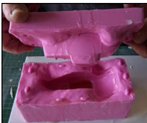
Pour a little resin over the "plug" part of mould. Carefully, push "plug" into base, aligning registration keys accurately.
