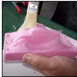
Dust the mould with talcum powder.
