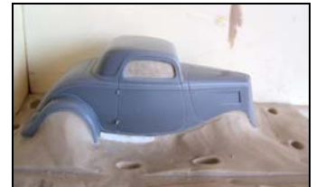
Embed the Model in clay on mould box base. Add holes for registration keys.
