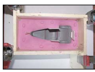
Rebuild mould box. Apply release agent.
