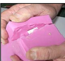
Build mould box. Measure, mix and pour silicone. Allow silicone to cure.
