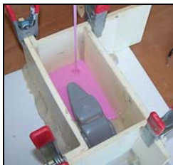
Build mould box. Measure, mix and pour silicone. Allow silicone to cure.
