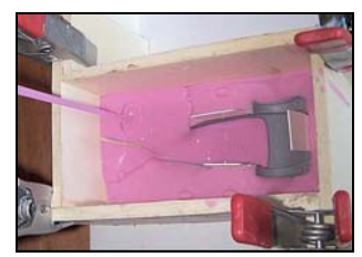
Measure, mix and pour second half of silicone. Allow to cure
